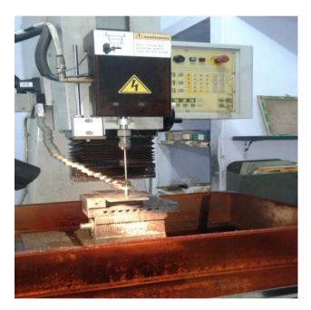
Figure 1: Electric discharge machine
